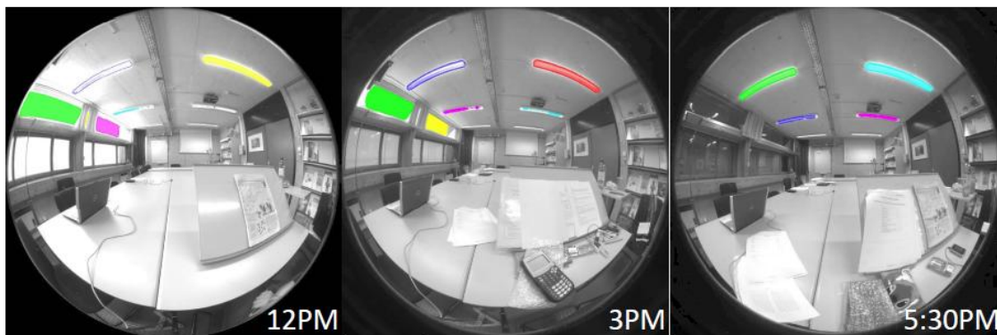
Glare sources are indicated with different colors and quantified by using 'Evalglare' (Wienold & Christoffersen, 2006).
