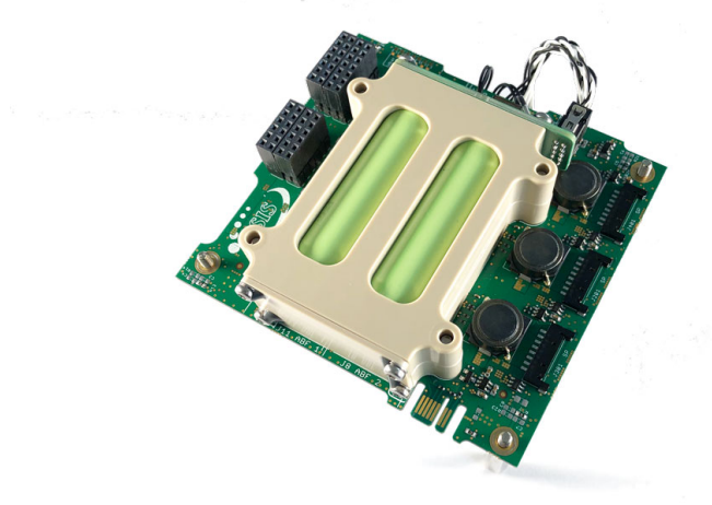
Figure 24: iEPS Electrical Power System from ISISpace, with the battery pack
