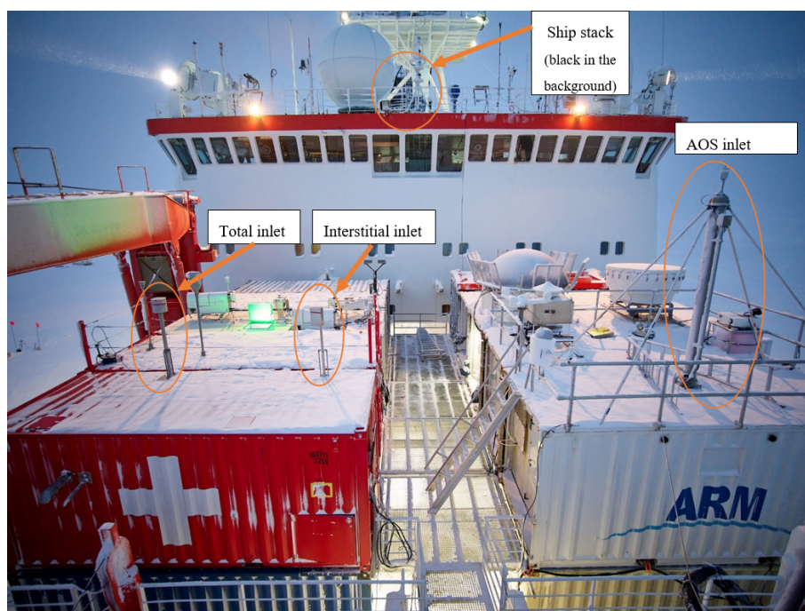
Figure A2. Bow of the ship during the expedition. In red with a white cross, the Swiss Container with its two inlets. The ARM measurements were performed on the port side of the ship in the white container at the front with a higher inlet. Photo credit: Michael Gutsche.
