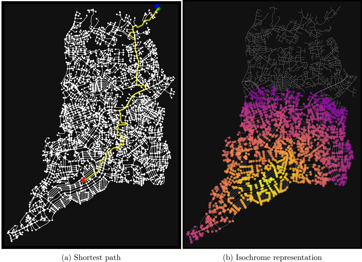
Figure 13 – Construction of the origin destination matrix with OSMnx Python toolbox. (a) illustrates the shortest path between a facility node location (red) and a chosen node (blue). (b) illustrates a time-distance isochrone around this same departing location. Both figures represent applications over the district commune of Yaounde 5
