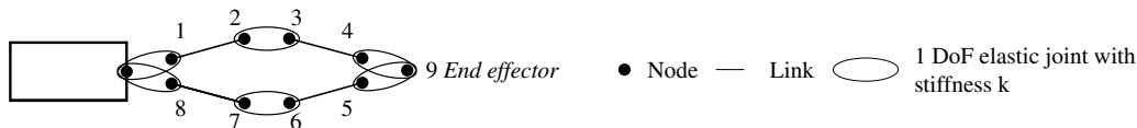
Figure 10. MSA model of a single diamond: A single diamond and its end-effector is modeled by nine nodes, four links, and six joints. We consider the links flexible and the joints elastic along one-DoF with stiffness k . The linear actuator is considered as the support and the floating node nine as the end-effector.
