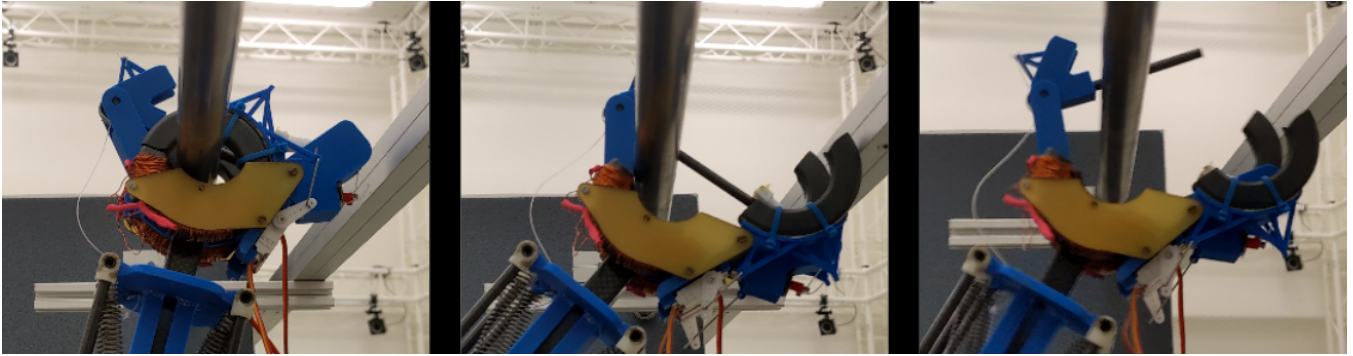
Fig. 5. Unperching Sequence. On the left, the mechanism configuration while recharging battery. In the middle, the split cores opened. On the right, the latch has been released, causing the bar to open and the UAV to fall.
