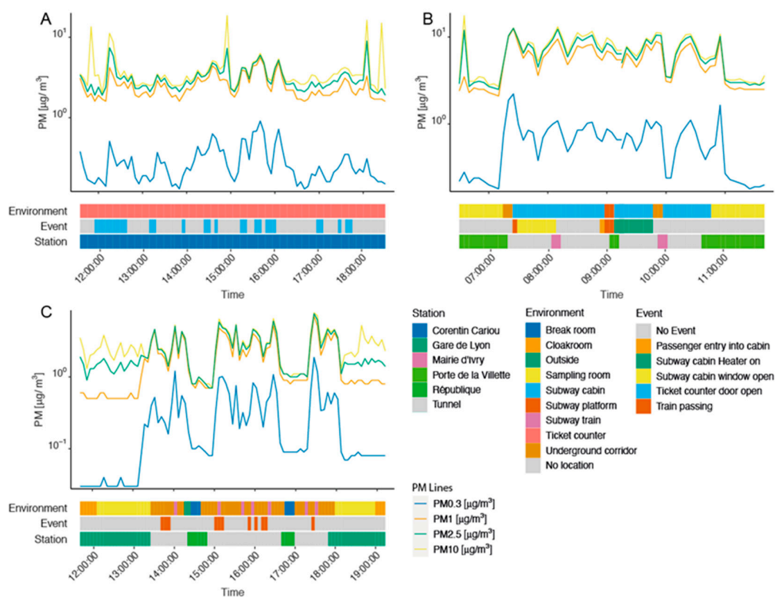
Figure 2. Real-time measurements of PM mass concentrations over the work shift in the PBZ for station agents (A) (11 October 2019), locomotive operators (B) (25 October 2019), and security guards (C) (7 November 2019).
