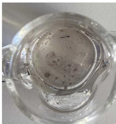
Figure S5.3. Photograph of the electrolyte after PEC testing showing the \text{WSe}_{\text{eds}} nanoflakes detachment
