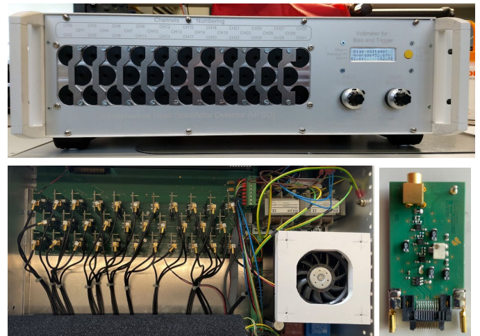
Fig. 9. Front-end (a) and internal (a) of a 32-channel module developed at LRS. One of the 32 fast-preamplifier board installed in the module (c).
