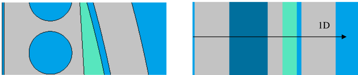
Figure 3.27. Heavy reflector assembly model (REFLE3) in Serpent2 (left) and CASMO5-VVER (right)
