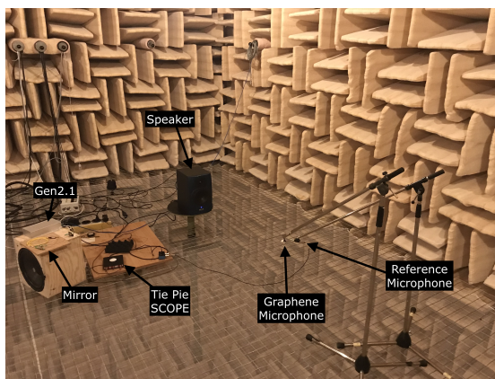
Figure 5.8: Setup mounted inside the anechoic chamber.
