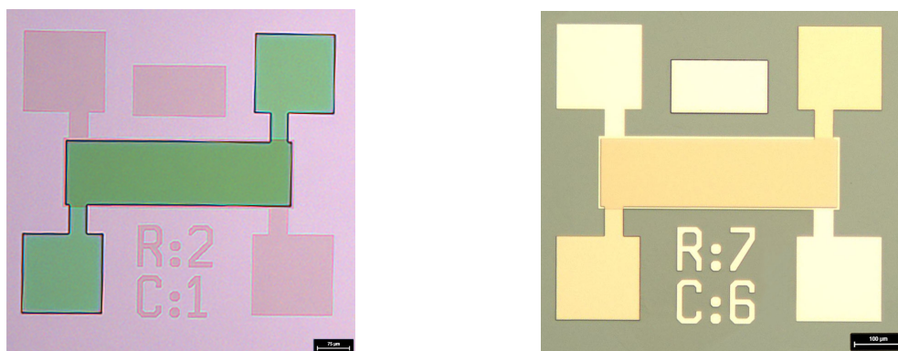
(a) Top electrode photolithography done on a wafer with 50 nm of \text{HfO}_2 . The alignment and exposure were performed with MLA150.
