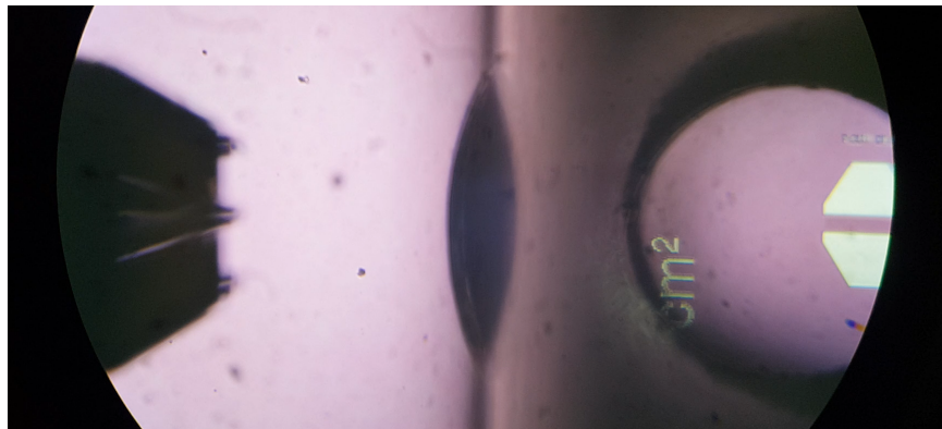
Figure 13: Microscope image of the probe (to the left), being getting near the pipetting cell. Also, the microscope could see in the channel to verify the alignment with the resonator (to the right).
