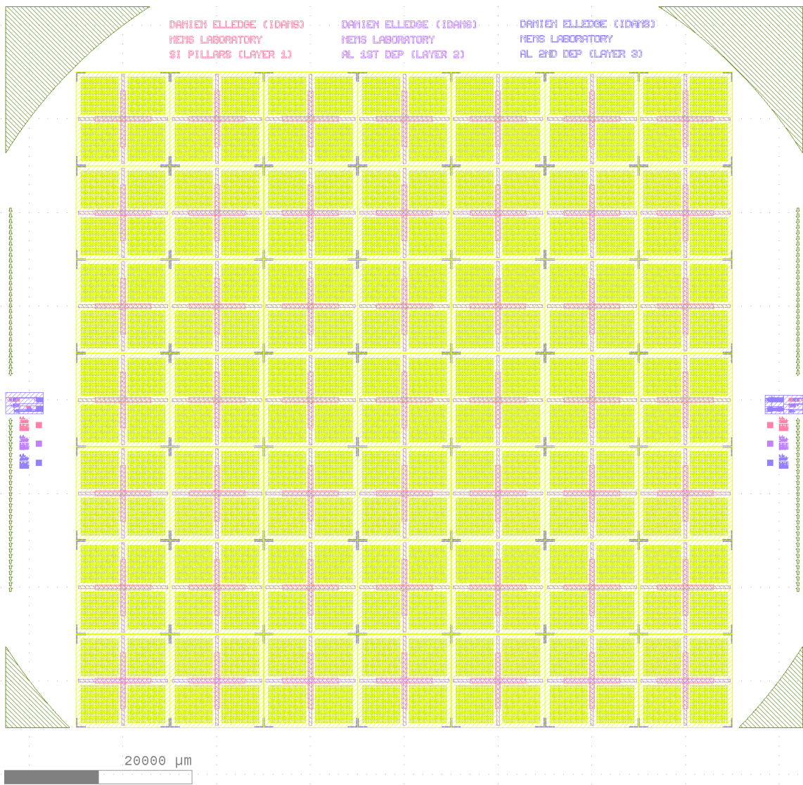
Figure 13: Design of the whole wafer with the 3 different masks used during the process flow
