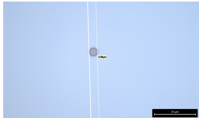
(b) Zoom in on a 5 \mu\text{m} diameter photoresist structure
