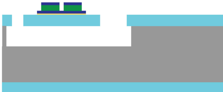
Figure 1: Cross section of one possible device. In blue the Pt, in yellow the Ti, in gray the Si, in light blue the SiN and in green the AlN. The dimension are not in scale and the image serves just to give an idea of the shape.
