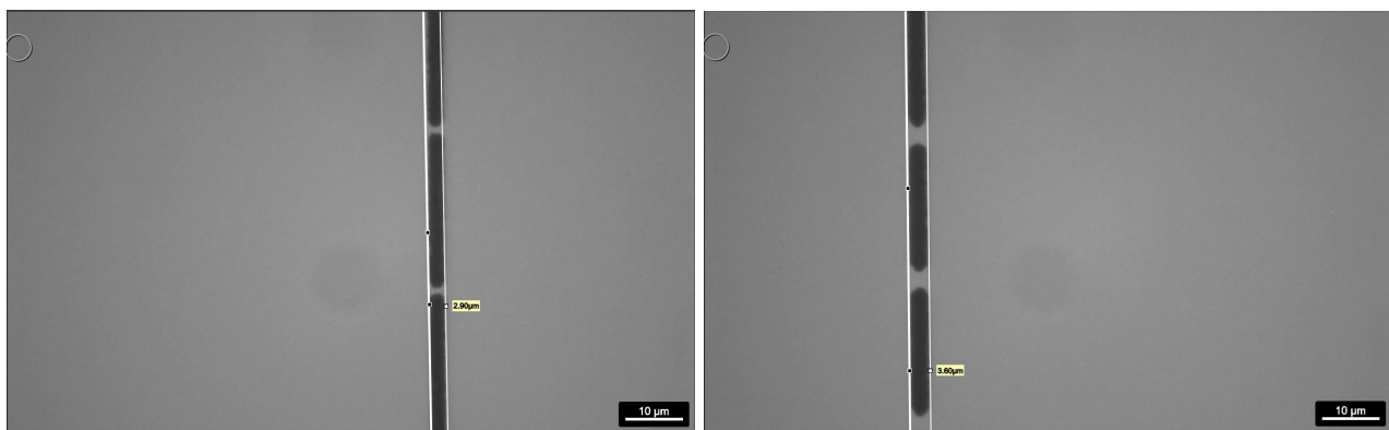
Figure 16: Comparison of two measurement for a 1500nm writing on a wafer after PECVD deposition at two different location
