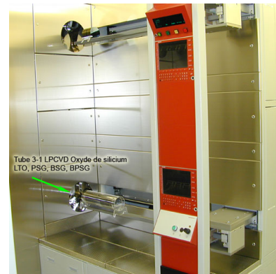
Figure 10: 3-1 tube for the LTO deposition [9]
