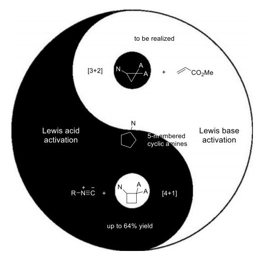
Figure 20. Synthesis of 5-membered cyclic amines from DA aminocyclopropanes or DA aminocyclobutanes.
