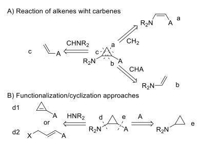
Figure 7. Retro-synthetic analysis of DA aminocyclopropanes.
