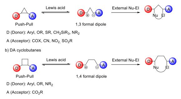
Figure 4. Activation and annulation of DA cyclopropanes and cyclobutanes.
