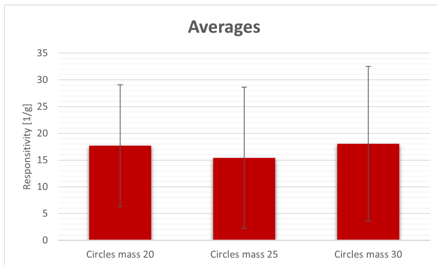
Fig. 17: Average measurements of device's responsivity with different circles mass sizes with the micro-ship clamped with glue.
