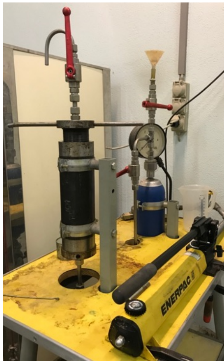
Figure 3.3 : Pressure column system.
