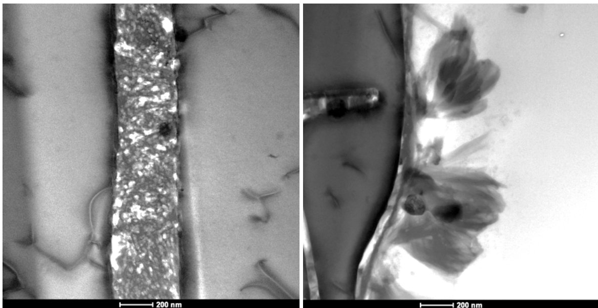
Figure 4.8 : In two neighbouring cracks, presence of (left) granular and (right) platey product.
