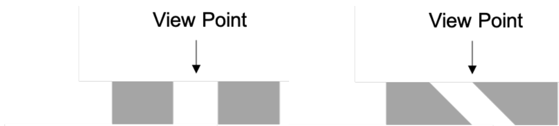
Figure 4.4 : Different crack orientations: The direction of electron beam (left) is suitable for analysis in contrast to (right).
