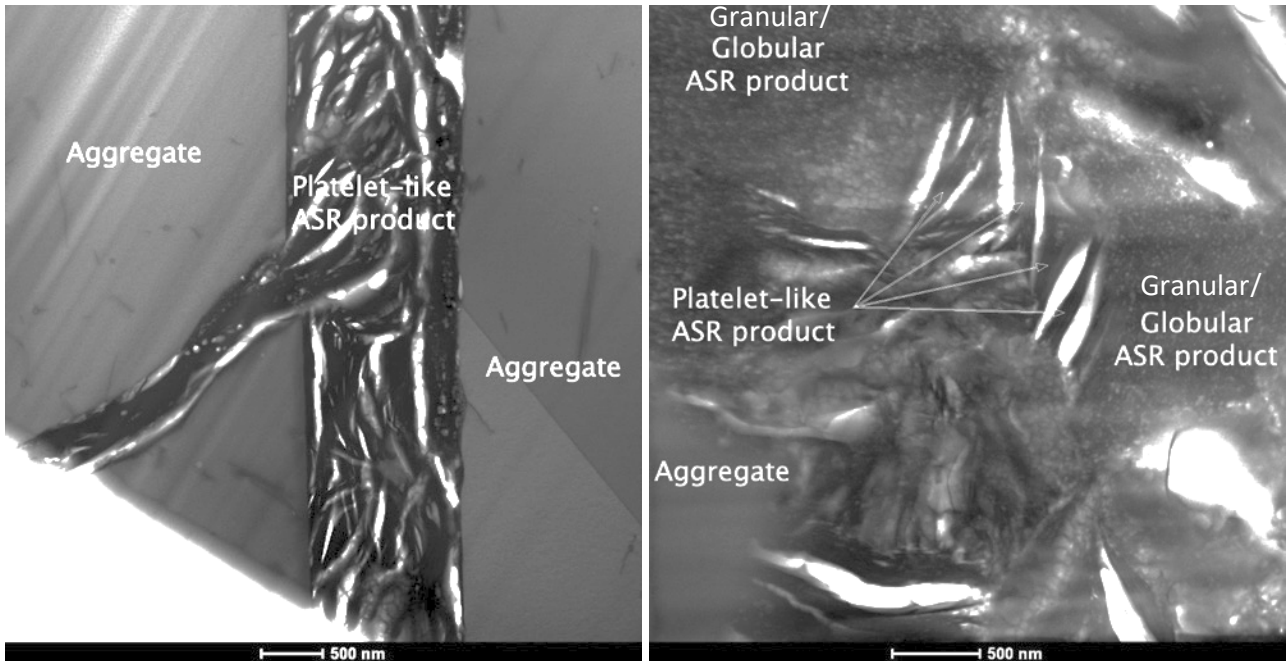
Figure 7.11 : Wall L1 showing platelet-like morphology (but amorphous) (left) and Wall L2 showing the intermixing of both granular/globular and platelet-like morphologies (right).
