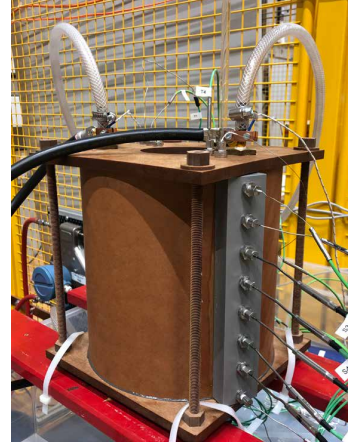
Figure 4: Vessel, instrumented with thermocouples, containing oil and a pair of PW and SW connected to a DC power source and DI WCU.
