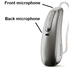
Figure 2.2: Example of hearing aid equipped with two omni-directional microphones: Phonak Audéo P.
