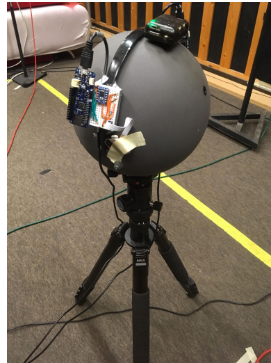
Figure 6.5: Artificial head equipped with the prototype, and mounted on the motor of the turntable.
