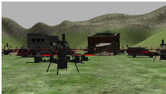
FIGURE 9. Screenshot of a collective search and rescue mission with a swarm of one hundred quadcopters in the Gazebo simulator. During the mission, the quadcopters take off from the ground and navigate towards a fictitious disaster scenario.
