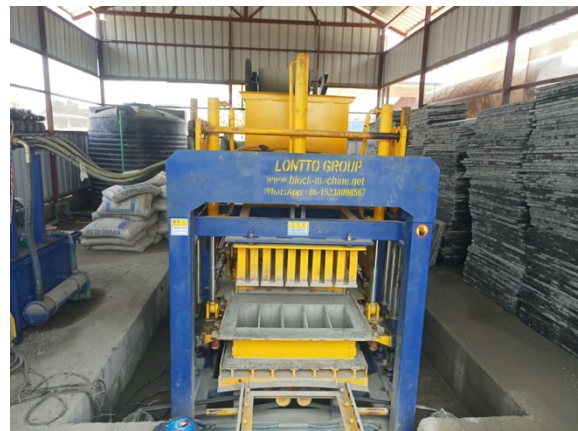
Mechanical production of cement block
