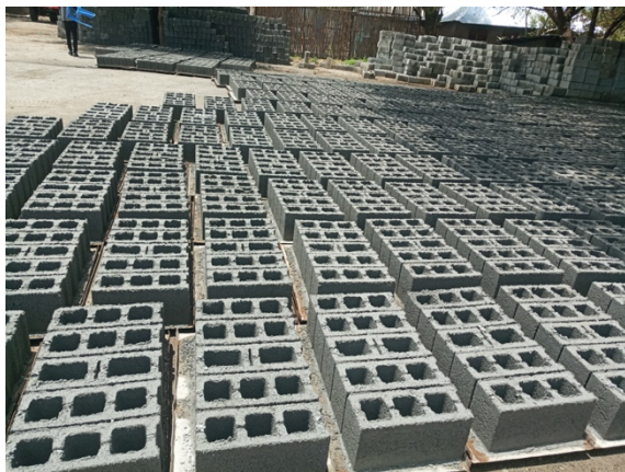
Cement block production
