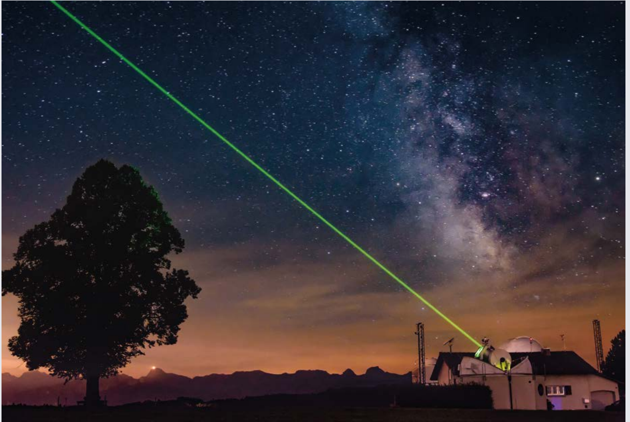
Laser beam transmitted from the 1-meter ZIMLAT telescope at the SwissOGS to measure the distances of artificial satellites with a mm-accuracy. (photo: AIUB, Emiliano Cordelli)
