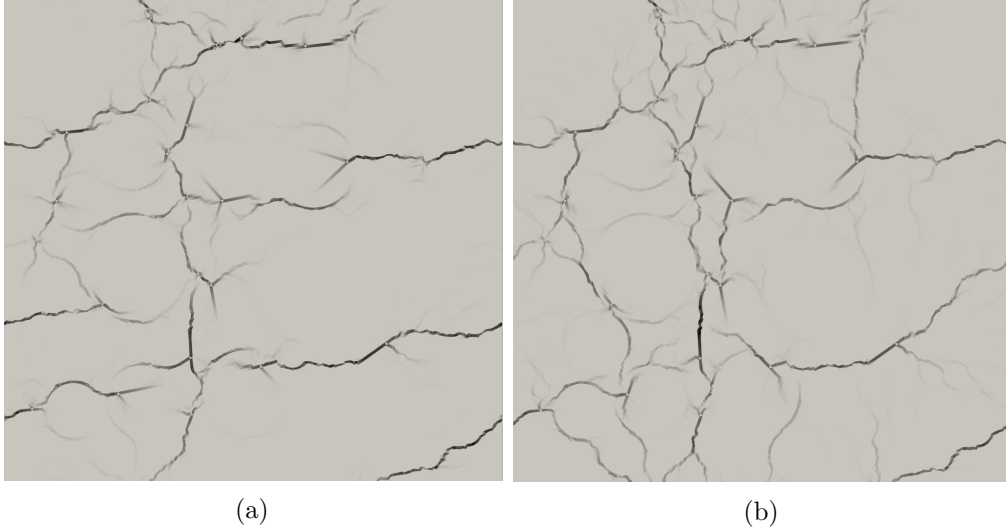
Figure 6.28: Crack opening maps of the RVEs at a) the bottom and b) the crest at the age of 70 years.
