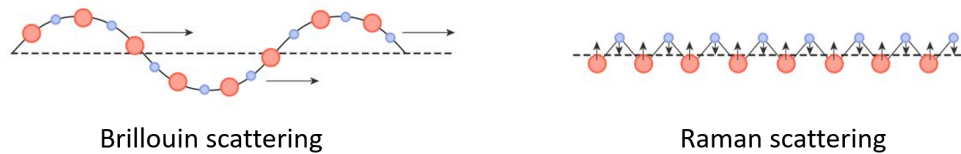
Figure 2.17 – Differences between the acoustic-like vibration in the left and the optical-like vibrations in the right.
