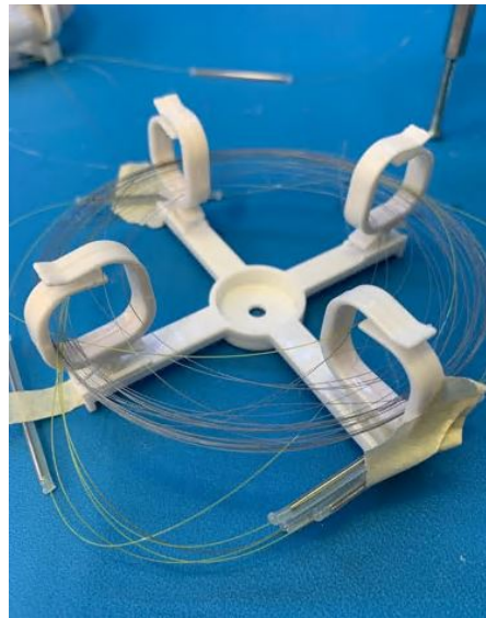
Figure 4.21 – Silicone-coated fibres in a stress-free holder.
