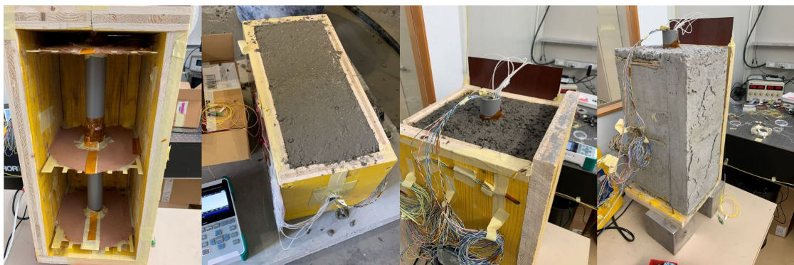
Figure 5.3 – Wood formwork before and after pouring concrete, and concrete block after a few days of curing.
