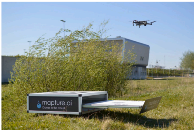
Fig. 7. Example of UAV recharging station (courtesy of Mapture.ai).
