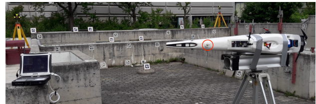
Figure 3. Lever-arm calibration camera to GNSS antenna, phase-center of which is represented by a tip of pin (red-circle).
