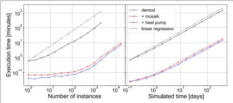
**Fig. 4** Measurement of execution time of a simulation of one day with increasing number of households (left side) and 32 households with increasing simulated time (right side)
