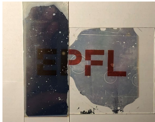
Figure 21 - Photograph of the 20 nm silver coating (on the left) compared to the nanoimprint-structured sample (on the right).
