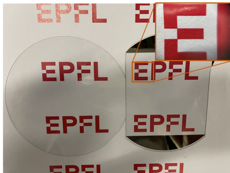
Figure 25 – Left: reference float glass and right: honeycomb micromesh with a linewidth of 2 \mu\text{m}
