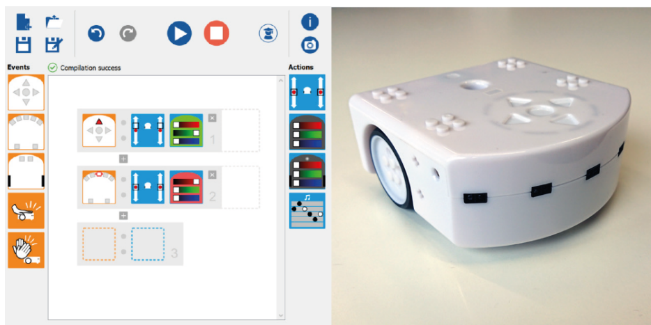
Fig.5 Illustration of proximity between the VPL programming interface and the Thymio robot. The figure illustrates the iconic representation of programming commands in the VPL programming platform (left). The icons were designed to be as close as possible to the characteristics of the Thymio robot (right).
