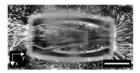
Figure 5.3 – Flow profile inside and around  $\mu$ jet engine a) Streamlines inside and around the  $\mu$ jet engine are visualized experimentally using fluorescent microparticles. Scale bar: 75  $\mu$ m
