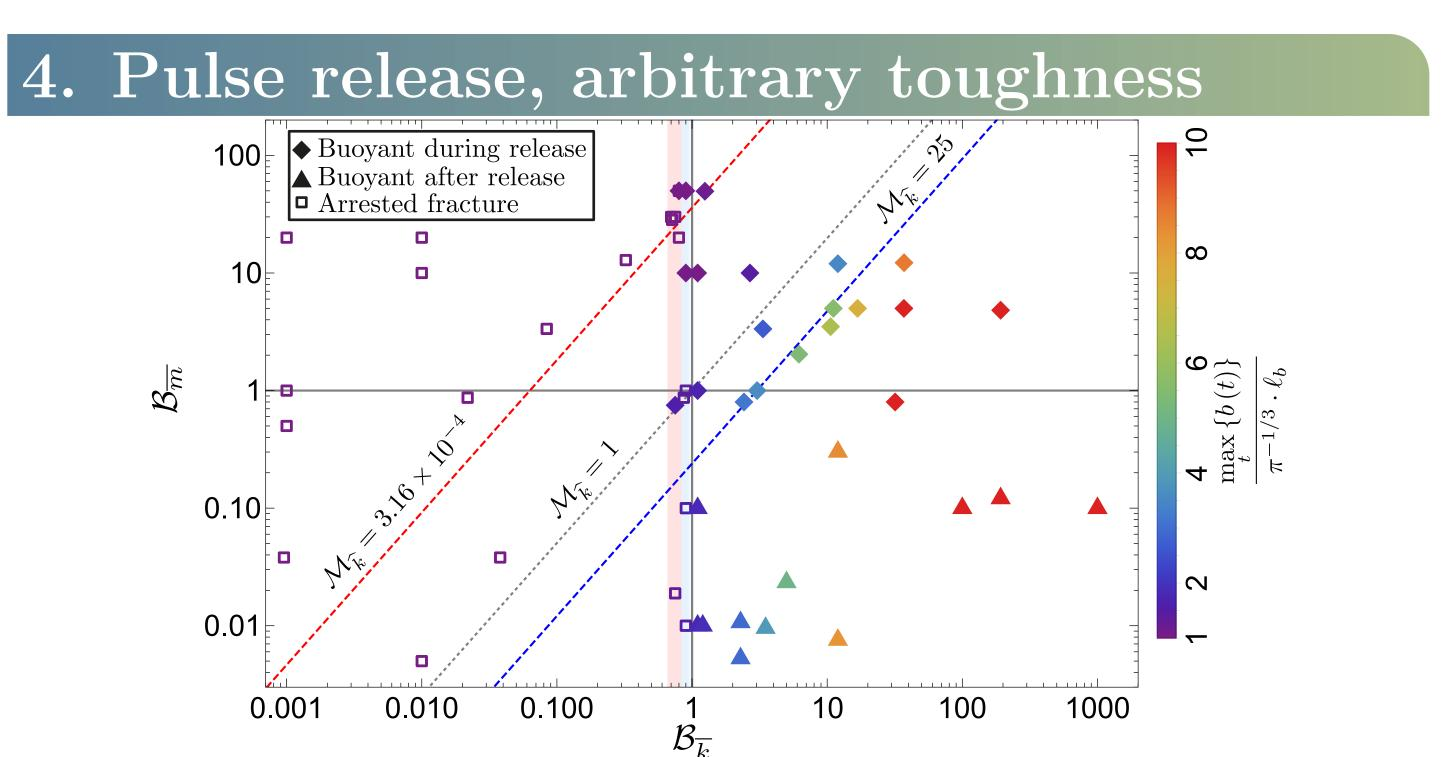
$\mathcal{B}_{\overline{k}}$  indicates if buoyant propagation establishes (full symbols). At late time, the head breadth approaches the zero-viscosity limit. The color code shows the fraction between maximum and limiting breadth. Various general shapes for the final buoyant crack exist, the shape is largely dominated by a combination of  $\mathcal{B}_{\overline{k}}$  (x-axis) and  $\mathcal{B}_{\overline{m}}$  (y-axis).
