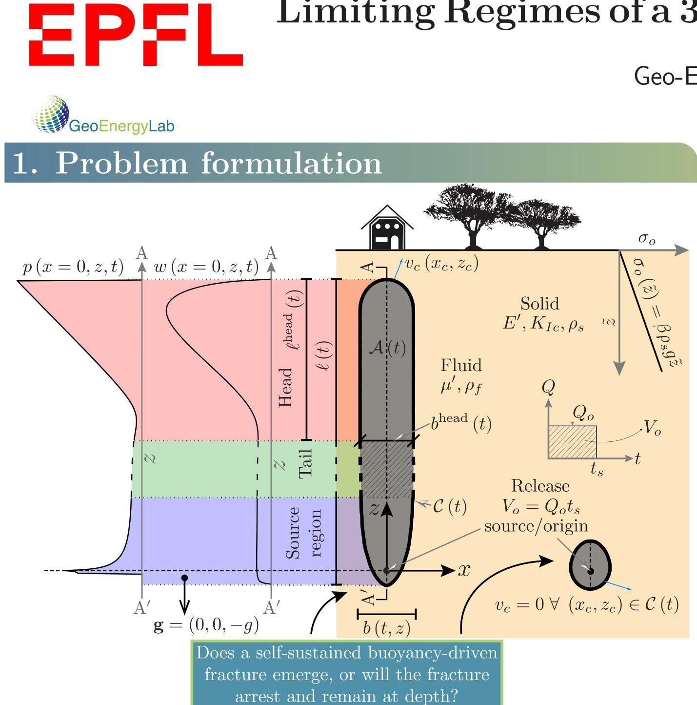
The problem of a planar mode I fracture assuming LEFM, no leak-off, and zero fluid-lag, is solved using PyFrac (Zia and Lecampion, 2020), an ILSA-based open-source solver. A scaling analysis reveals three main dimensionless coefficients
