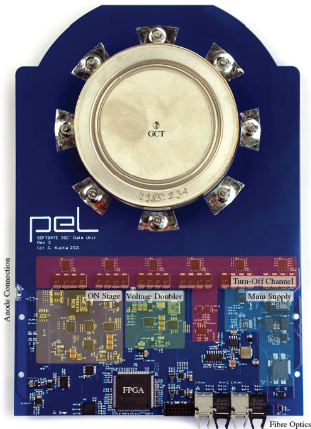
Fig. 5. Photo of the gate unit designed for soft-switching application.
