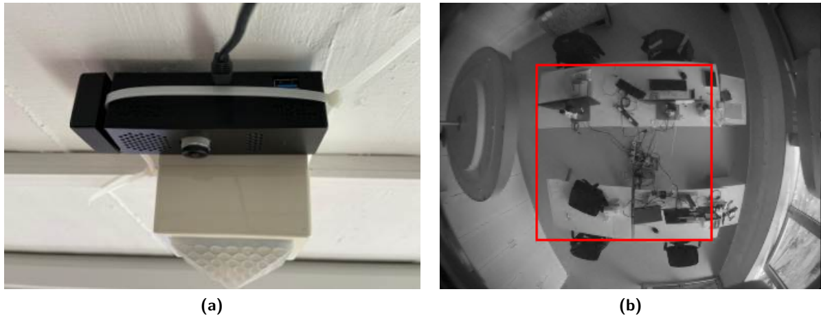
Figure 4.5 – a) Glare Meter installed on the ceiling; b) greyscale image captured by the sensor: the average work plane illuminance is estimated starting from the average luminance of the pixels within the red rectangle (which can be adjusted via software according to the requirements).
