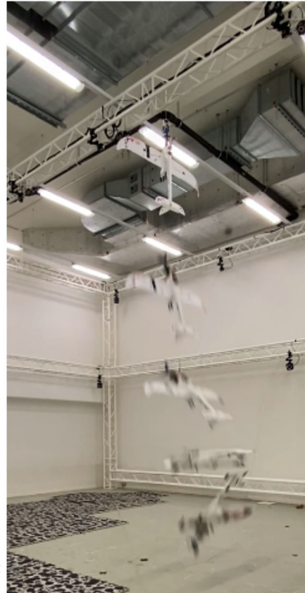
Figure 8. Results of the drop test. On the left are plots of the height and velocity of the aircraft as it falls. Gaps in the data are due to the motion capture cameras losing track of the markers.
