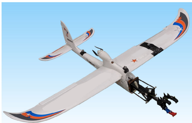
Figure 1. Photograph of aircraft with perching claw on front.
