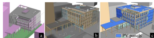
Figure 2. (a) Building-Energy Model, (b) Solar Energy Model and (c) Potential active surfaces (in blue)
