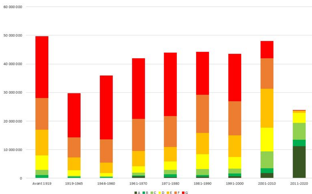
Figure 1: Energy reference area in m 2 per construction period and energy class (for energy thresholds, see Table 1); the year 2015 (source: our estimations, using data from the SFOE. See Appendix C)
