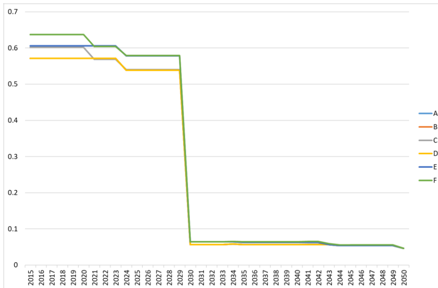
Figure 19: Plant specific CO 2 emissions in t CO 2 per ton clinker – Low EPB with CCS and ETS price floor in 2030. Source: Own Figure.
