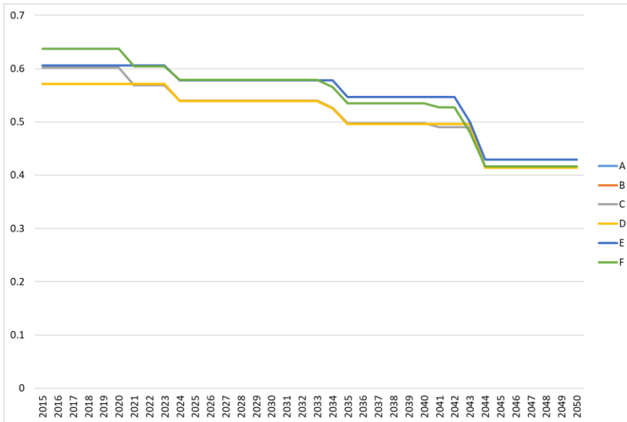
Figure 15: Plant specific CO 2 emissions in t CO 2 per ton clinker – Low EPB. Source: Own Figure.
