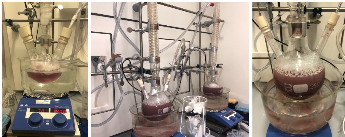
FIGURE 2.11 – pNIPMAM coating of AuNRs set-up. On the left, the polymerization is ongoing. In the first 30 min the suspension should change from transparent to this strawberry milkshake color. In the middle, a picture of 2 batches after polymerization. It is also possible to observe the reflux column in the middle neck, the N 2 flow connected with a Pasteur pipette on the right neck and on the left neck I connected a syringe tip through the silicon cap to allow the regulation of pressure. On the right, a zoom-in picture of the reaction suspension once the reaction is over.
