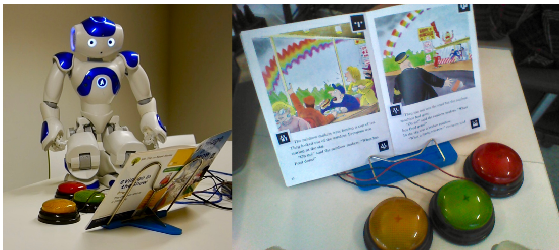
Figure 4.1 – CoReader platform; Left image shows the robot with the book and buttons; Right image shows the view from the robot's bottom camera looking at the book readable to robot through ARTags.
