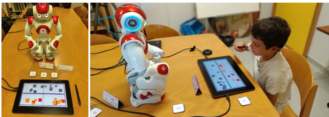
Figure 5.3 – The experimental setup when robot is the instructor and child is the manipulator.
