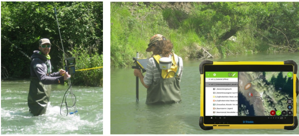
Figure 3: Field equipment used for surveying: The handheld Acoustic Doppler Velocimeter FlowTracker by SonTek (left), field tablet Trimble T10 and GNSS antenna Trimble R2 (right)
