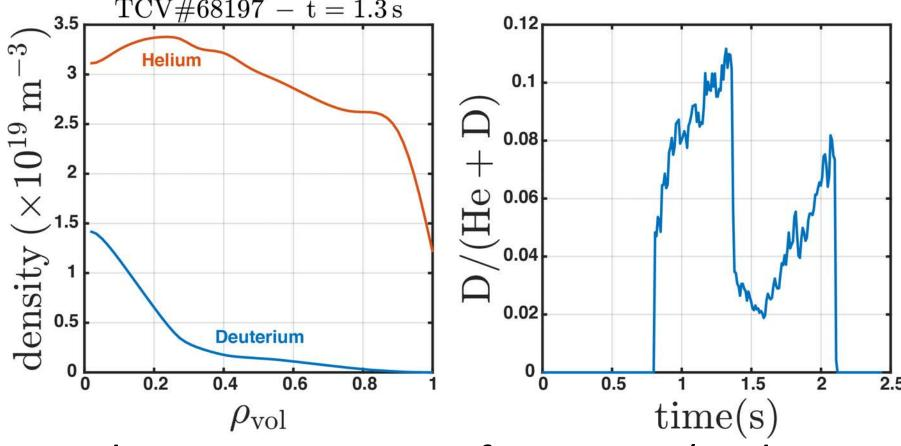
• Helium concentration from CXRS (preliminary) Absolute emission intensity of He II n=4-n=3 transition at  $\lambda=4686$  Å measured. 'Passive' emission subtracted (NBI glitches). He III density estimated from 'active' signal, and collisional-radiative calculations for the NBI evolution. Linear relationship with total injected flux.
