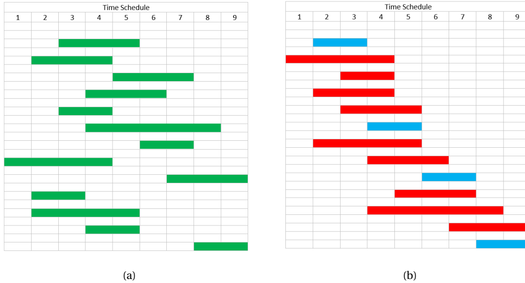
Figure 3.2 – The activity scheduling problem (left) and its proposed Greedy optimal solution (right) which sorts all activity by earliest finishing time and then perform a Greedy choice at each stage based on this criteria. The chosen ones are in blue and the eliminated choices are in red.
