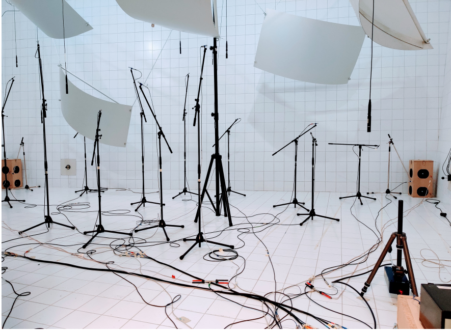
Figure 7.16 – Experiment set-up with 2 Electroacoustic Absorbers at the corners and 15 randomly placed microphones in the room.
