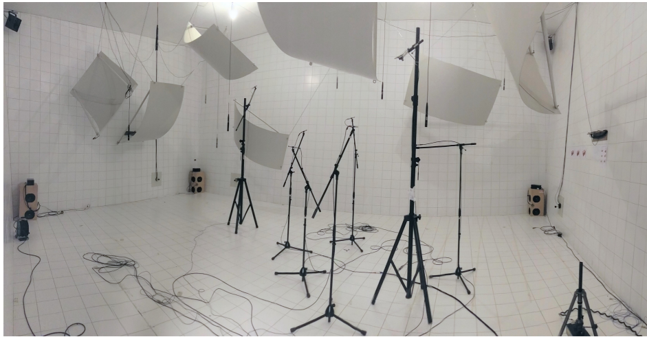
Figure 6.9 – Overall experiment set-up for sound field reconstruction with the Electroacoustic Absorbers.
