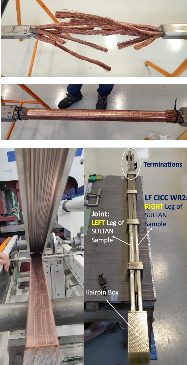
Fig. 4. Some pictures of the main manufacturing steps for the inter-layer joint. From top to bottom: the two cable ends after Cr-coating removal and cut with staggered geometry; crimping of the Cu sleeve; lamination to the final geometry and dimensions; closing of steel box with grooves for He circulation (left); final joint sample (right), after assembly of the bottom hairpin box.
