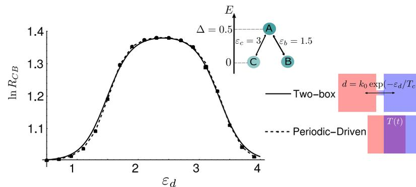
**Figure 6.** The logarithm of the selection strength as a function of the critical barrier  $\epsilon_d$  for a three-state, two-box model (solid line), as sketched in the inset, and for a time-periodic driven three-state system (dashed line). These two paradigms are qualitatively and quantitatively equivalent to determine non-isothermal selection of states.
