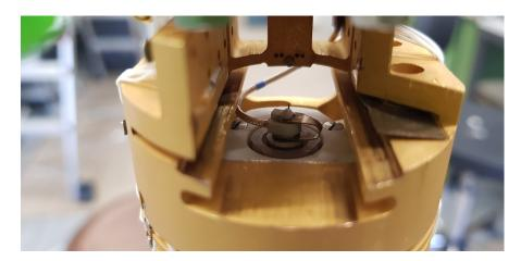
Figure 2.6: Novel tip holder installed in the STM head: The tip holder (white) is held in place by a metallic spring, which had equally been used before in conjunction with the old tip holder. In the background, the flexible RF cable leading up to the STM tip can be seen.
