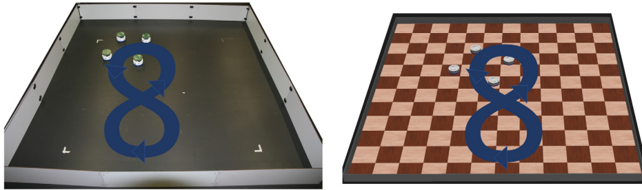
Fig. 5. Four Khepera IV robots in a diamond formation in the 3 m \times 3 m arena superimposed by the 8-shape they are tasked to drive in reality (left) and Webots (right).
