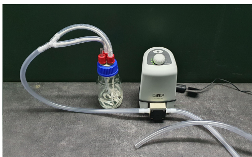
Figure 4.5 – Electric pump and ethanol recipient used as gas source.
