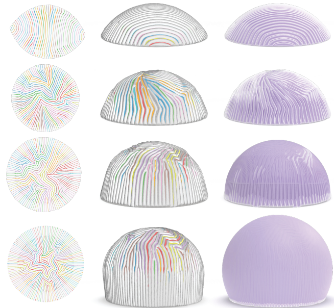
Fig. 13. Not all shapes can be inflated from a single patch. For increasingly larger parts of the sphere, metric distortion eventually exceeds the bounds realizable by the limited air channel contraction, leading to increasingly larger deviations from the target shape.
