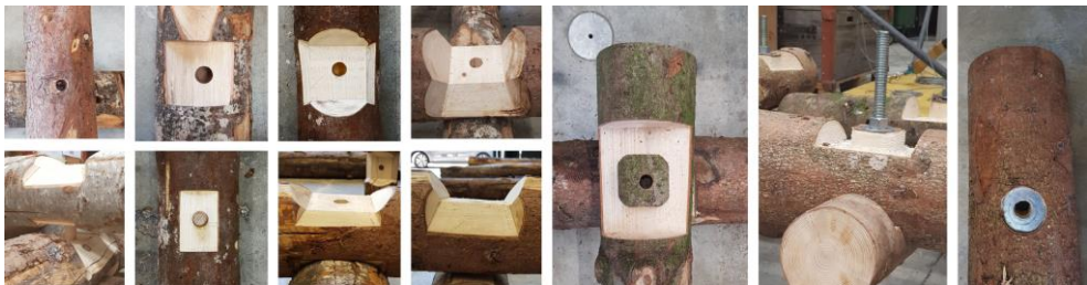
Fig. 12 Raw-wood cross-lap joints vary from a single dowel, surface flattening to conical cuts.
