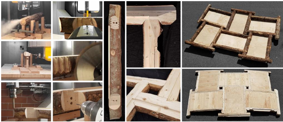
Fig. 4 Fabrication of the panel braced Nexorades is tested using raw wood and translation method.
