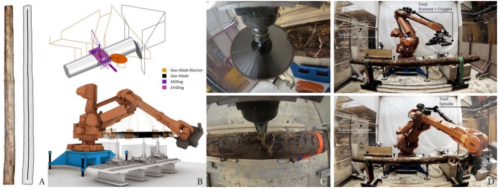
Fig. 13 Fabrication steps: A) central-axis, B) tool-path, C) cutting process, D) scanning and cutting.
